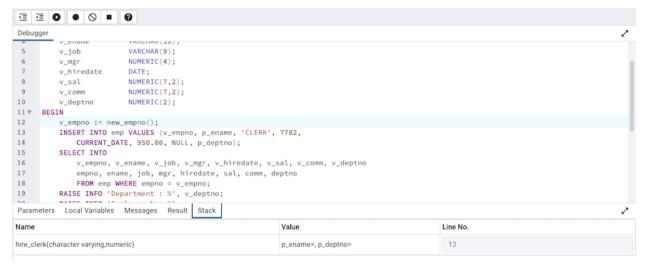
Select a caller to change focus to that stack frame and display the state of the caller in the upper panel.
