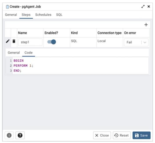
Use the context-sensitive field on the step definition dialog's *Code* tab to provide the SQL code or batch script that will be executed during the step:
