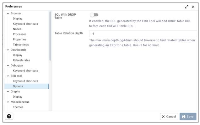
• When the *SQL With DROP Table* switch is set to *True*, the SQL generated by the ERD Tool will add DROP table DDL before each CREATE table DDL.
