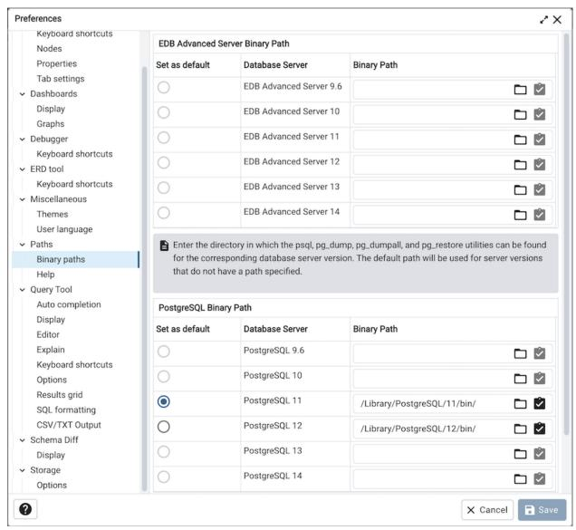
Use the fields on the *Binary paths* panel to specify the path to the directory that contains the utility programs (pg\_dump, pg\_dumpall, pg\_restore and psql) for monitored databases:
