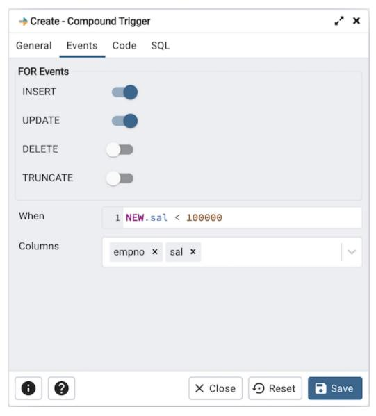
Use the fields in the *Events* tab to specify how and when the compound trigger fires:
