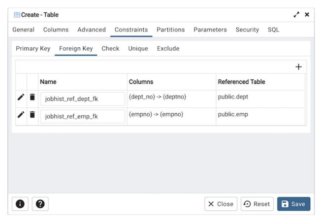
To add a foreign key constraint, select the *Foreign Key* tab, and click the *Add* icon (+). To define the constraint, click the *Edit* icon to the left of the *Trash* icon. A dialog similar to the *Foreign key* dialog (accessed by right clicking on *Constraints* in the *pgAdmin* tree control) opens.
