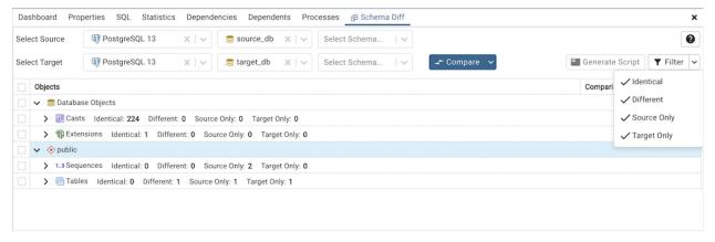
Click on any of the database objects in the object comparison panel to display the DDL Statements of that object in the DDL Comparison panel.
