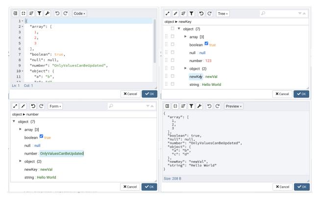
*Code Mode*: Provides way to format & compact json data. Also provides ability to repair json data by fixing quotes and escape characters, removing comments and JSONP notation and turn JavaScript objects into JSON.
