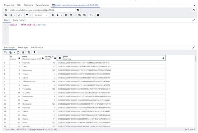
To modify the content of a table, each row in the table must be uniquely identifiable. If the table definition does not include an OID or a primary key, the displayed data is read only. Note that views cannot be edited; updatable views (using rules) are not supported.
