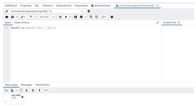
3. You can observe the *Notification* tab in the first *Query Tool* session where it shows the Recorded time, Event, Process ID, and the Payload of the particular channel.
