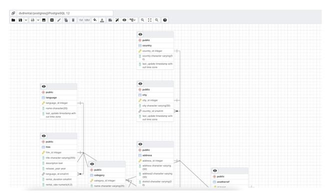
You can open multiple copies of the ERD tool in individual tabs simultaneously. You can also generate an ERD from a database, schema or a table.
