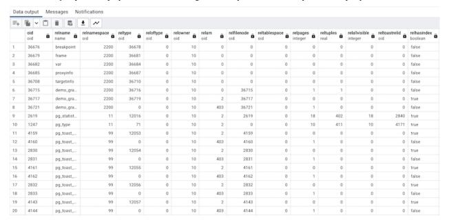
The Data Output tab displays the result set of the query in a table format. You can:
