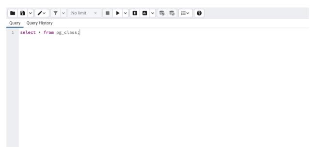
To use autocomplete, begin typing your query; when you would like the Query editor to suggest object names or commands that might be next in your query, press the Control+Space key combination. For example, type "SELECT \* FROM" (without quotes, but with a trailing space), and then press the Control+Space key combination to select from a popup menu of autocomplete options.
