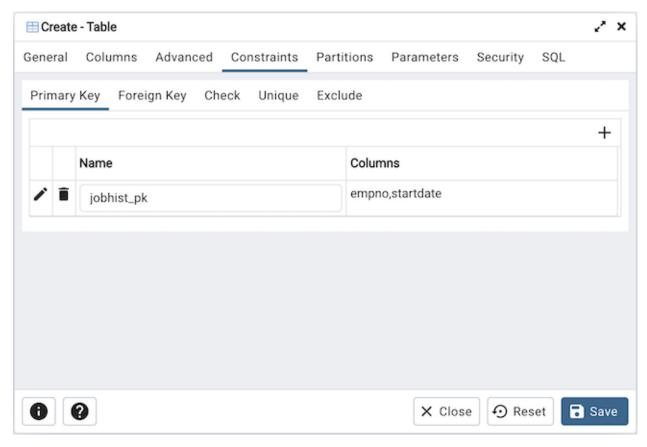
Use the fields in the *Constraints* tab to provide a table or column constraint. Optional constraint clauses specify constraints (tests) that new or updated rows must satisfy for an *INSERT* or *UPDATE* operation to succeed. Select the appropriate constraint type by selecting one of the following tabs on the *Constraints* panel:
