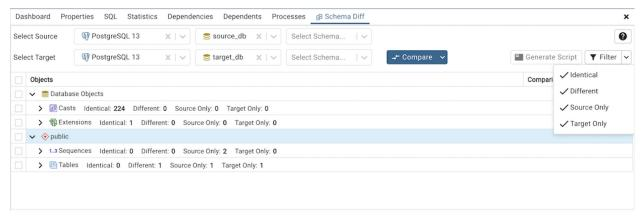
Click on any of the database objects in the object comparison panel to display the DDL Statements of that object in the DDL Comparison panel.
